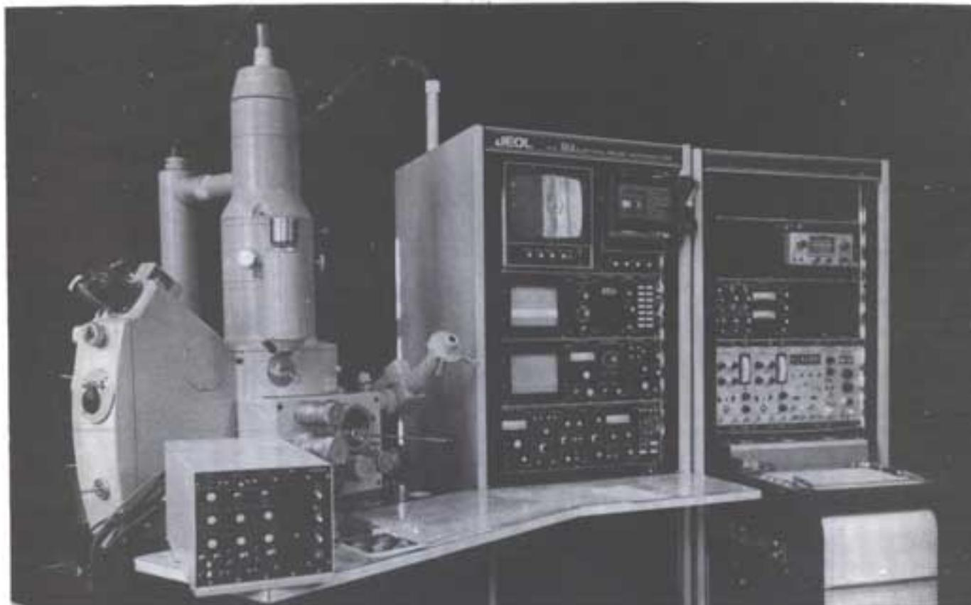
Scanning electron microscope/electron microprobe analyser used for examination and chemical analysis of minute areas of solid surfaces down to 2-3 microns in diameter. This photo illustrates the complexity and sophistication of modern analytical equipment. (Photo: IIR5)
